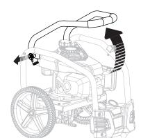
Install the trigger handle holder, spray wand holder, and hose storage (see page 7).
