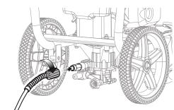
Completely uncoil and straighten high pressure hose to prevent kinks.
