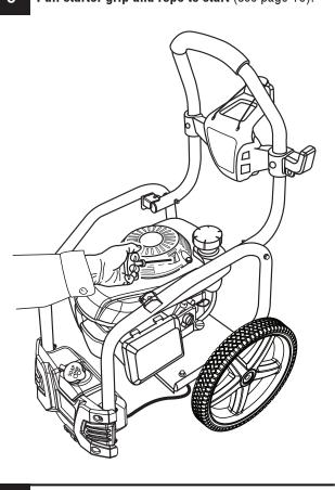
Allow engine to run for several seconds, then move choke to RUN position (see page 10).
